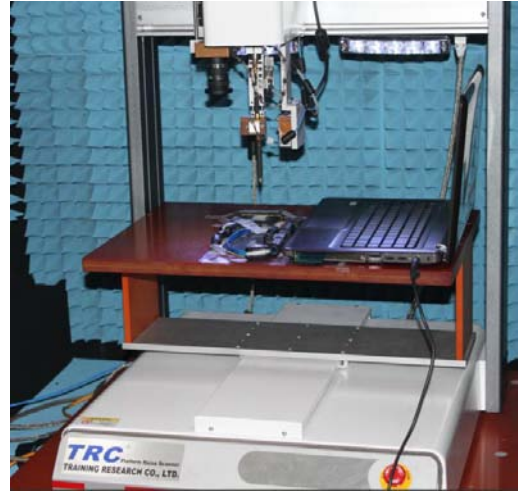
Fig. 4. Noise coupling analysis with surface scan measurement
